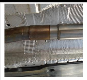
Step 3. Install your new system by first attaching the Inlet Assembly to the catalytic converter outlet. Lightly tighten the slip clamp to hold the component in place.
