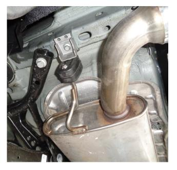
Step 2. Next, Disengage all welded hangers from the rubber insolators. The exhaust system can now be removed. Retain all fasteners and insulators as they will be needed to mount your new MAGNAFLOW system.
