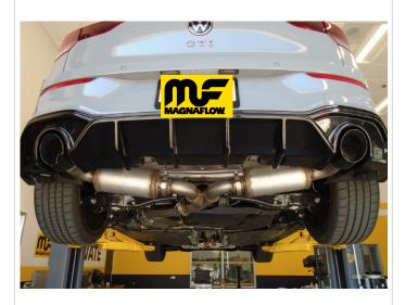
Step 6. Install both tip assemblies with the hanger first, and then connect to the Y-Pipe Assembly using a 2.5" V-Band Clamp. Center the tips, and then fully tighten all clamps starting in the rear, and proceeding to the front of the vehicle. Inspect all fasteners after 25-50 miles of operation and retighten if necessary.
