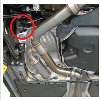
Step 4. Install the NDT Assembly using a 3" V-Band Clamp. Lightly tighten the slip clamp to hold the component in place. Using the supplied rubber isolater, Utilize the additional factory hanger circled in red.
