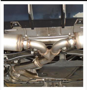
Step 5. Install the Y-Pipe Assembly using a 3" V-Band Clamp and loosely tighten to hold the component in place.
